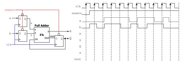
Provide the State Diagram (any representation), the Excitation Table, and the Excitation equations of the following Finite State Machine: (12 pts)
